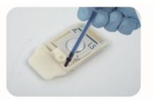
**Step 2:** Fill the inlet with sample to the fill mark and slide the cap to seal the inlet
