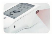
**Step 1:** Scan the barcode on the cartridge pouch and take out the cartridge from its pouch
