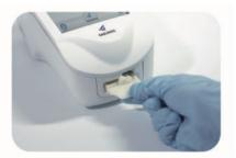
**Step 3:** Insert the cartridge into the analyzer until it clicks. Wait for the results
