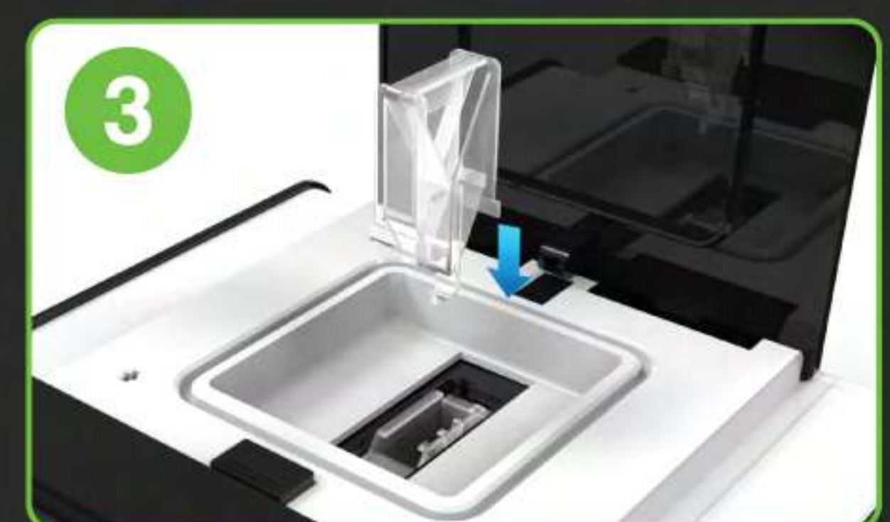
3 Insert the reagent pack and the result will be appeared in less than 5 minutes.
